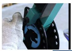
Adjust the height of the arm so that the lifting cord is directly above the middle of the edge of the windscreen.
