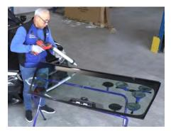
Prep the new glass and attach the suction cup frame. Positioning the frame over the side of the windscreen allows you to rotate the glass off the stand.
