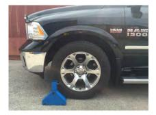
Find a level space, ensuring that there is enough room to walk around the vehicle with the piece of glass attached to the winch. Place the support arm wheel plate in front of the tyre that you will be using to hold the plate. When installing a panoramic roof use the rear wheel.
