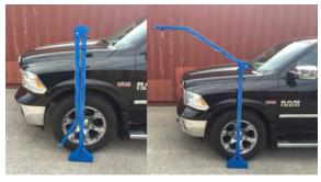
Insert the support arm and tighten the two screws in the wheel plate upright. Unfold the arm taking care not to touch the vehicle. Beware of any pinch points when unfolding the arm.
