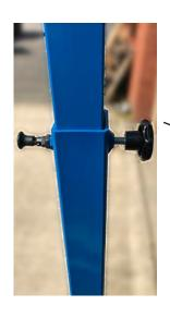
Once you have achieved your desired height using the lower vertical support ensure that the spring pin is correctly located and tighten the large security knobs to ensure the risk of a sudden drop is minimized.
