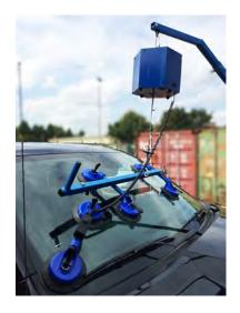
Place the suction cup frame on the glass and secure correctly. The frame should be in the middle of the glass. The higher the frame is on the glass the more inclined the glass will be.
